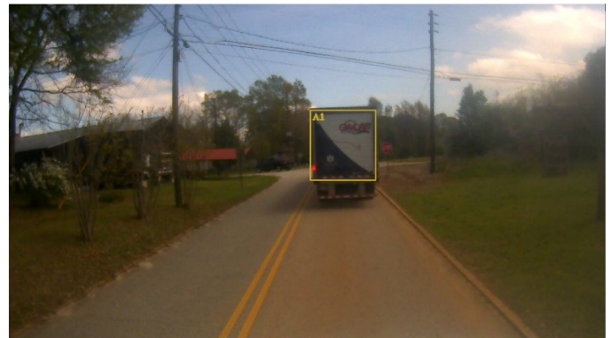
Figure 3: Example of Bounding Box Provided by YOLO
